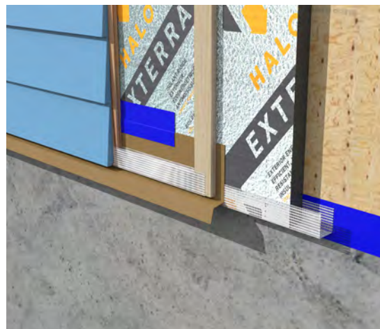
Foundation transition detail without trim board
